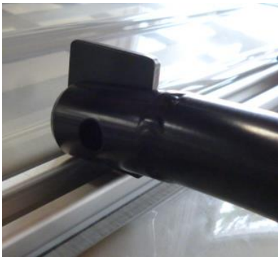
Figure 2: Surf Pole Positioned on "L" Brackets
