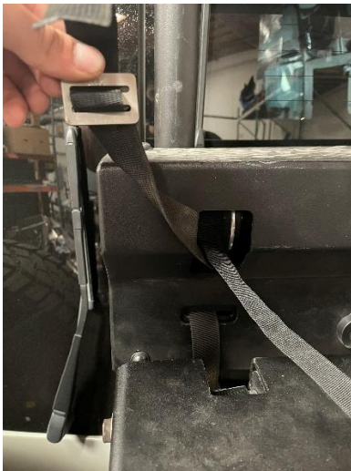
Figure 49: Webbing Anchor Pulled Through Pulley Holes
