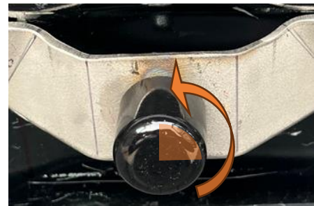
Figure 44: Unscrew Bump Stop 1/4 Turn to Increase Engagement
