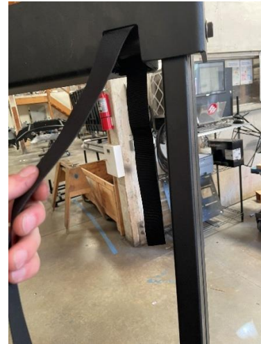
Figure 12: Threading Webbing Through Upper Tray Pulleys
