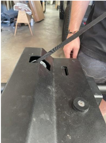
Figure 11: Threading Webbing Through Power Box Cover
