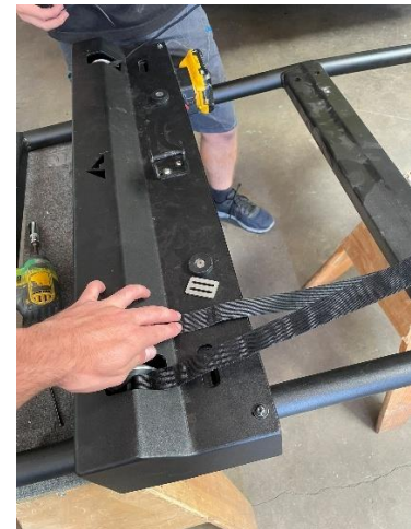
Figure 13: Bringing Webbing Back to Power Box
