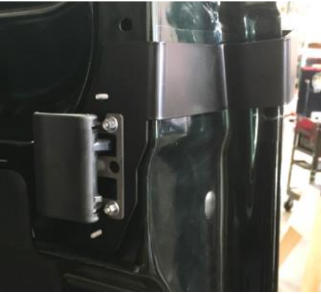
Figure 26: Upper Inner Passenger's Side Bracket Installed
