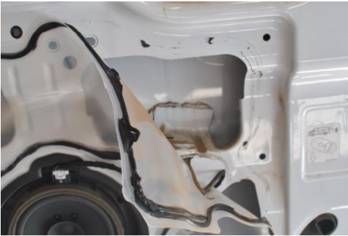
Figure 27: Inner Door Liner Peeled Back for Access
