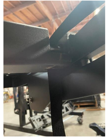
Figure 50: Webbing Threaded Over Pulley and Through Upper Tray Slot
