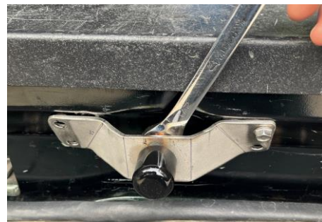
Figure 45: Tightening Jam Nuts on Rubber Bumper
