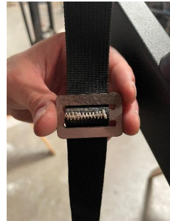
Figure 51: White Stitching Position on Webbing Anchors
