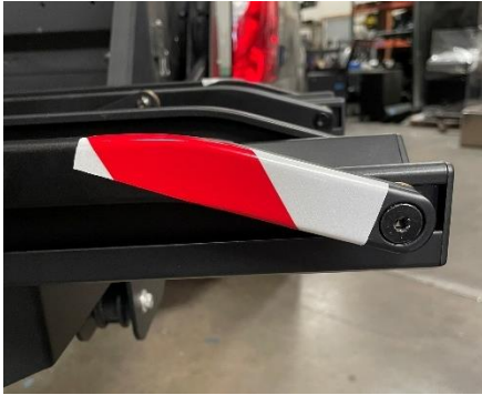
Figure 46: Reflective Tape Installation
