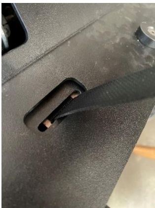
Figure 17: Webbing Anchor Installed Through Power Box Slit
