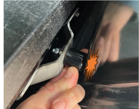
Figure 43: Bump Stop Adjustment to Passenger Door
