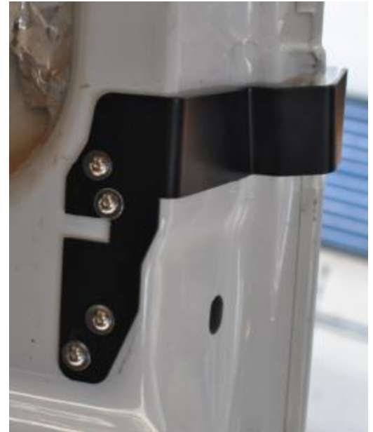
Figure 29: Installed Inside Upper Bracket without Factory Handle
