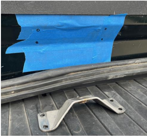
Figure 40: Pilot Holes Marked
