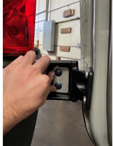
Figure 22: Lower Backing Plate Insertion
