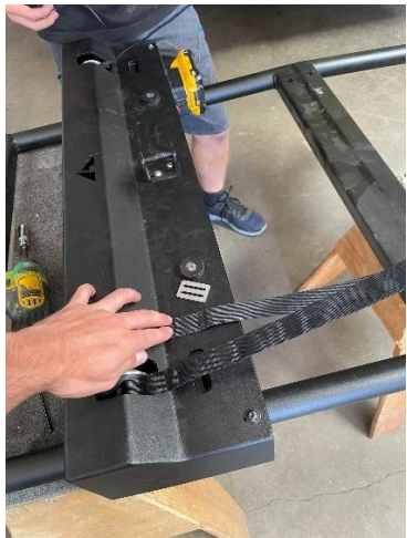
Figure 10: Bringing Webbing Back to Power Box
