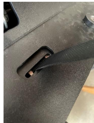
Figure 14: Webbing Anchor Installed Through Power Box Slit
