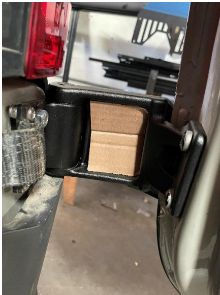
Figure 26: Cardboard to Push Bolts Out on Lower Hinge
