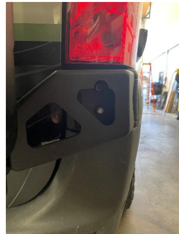
Figure 28: Heavy Duty Lower Bracket Mounting
