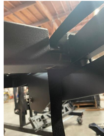
Figure 36: Webbing Threaded Over Pulley and Through Upper Tray Slot
