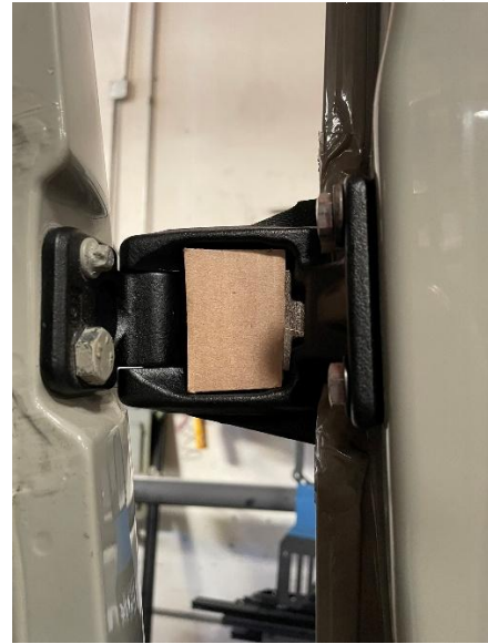
Figure 27: Cardboard to Push Bolts Out on Upper Hinge
