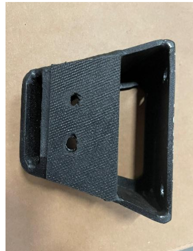
Figure 18: HD Upper Bracket with Foam Tape
