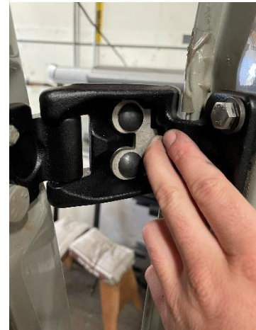
Figure 23: Upper Backing Plate Insertion
