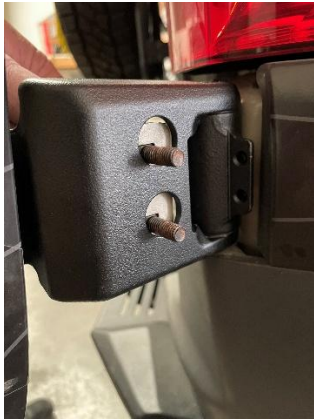
Figure 24: Lower Hinge Bolt Routing
