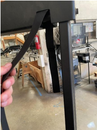
Figure 9: Threading Webbing Through Upper Tray Pulleys
