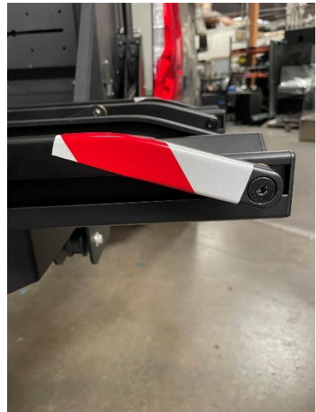
Figure 32: Reflective Tape Installation
