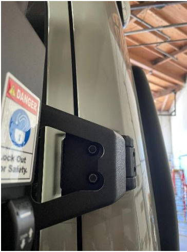
Figure 29: Heavy Duty Upper Bracket Mounting
