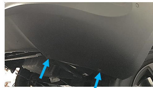
Figure 6: (2X) Plastic Rivets on Underside of Bumper
