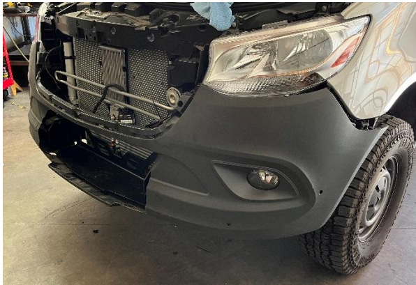
Figure 35: Loosely Installed Factory Front Bumper
