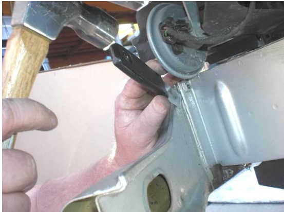
Figure 12: Releasing the Stock Steel Bumper from the Vehicle Using a Putty Knife and Hammer
