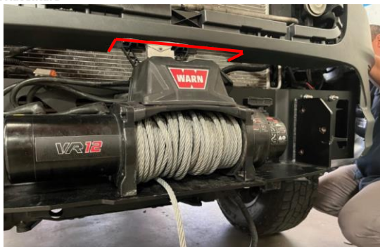
Figure 28: Winch Controller Relief Example
