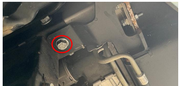
Figure 21: Installed Factory Crossmember Bolt Thru Winch Tray
