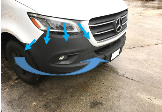
Figure 8: Removing Plastic Bumper
