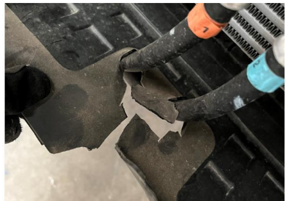
Figure 15: Air Flow Skirt Cut for Removal
