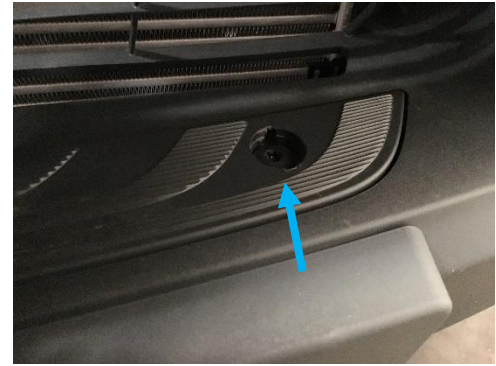
Figure 10: Front Bumper Step with Plastic Cap Removed
