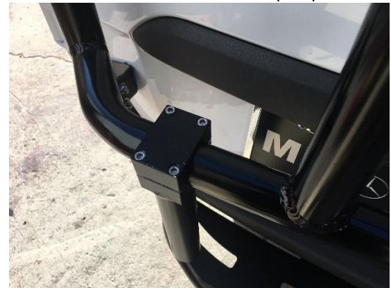
Figure 7: Bolt-On Supports Loosely Bolted to Lower Crossmember
