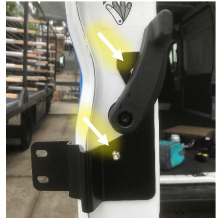
Figure 12: Inner Driver Door Bracket Installed
