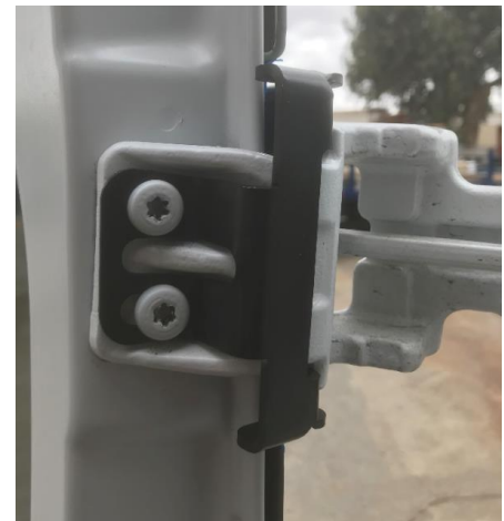
Figure 7: Inside View of Installed Upper Hinge Bracket
