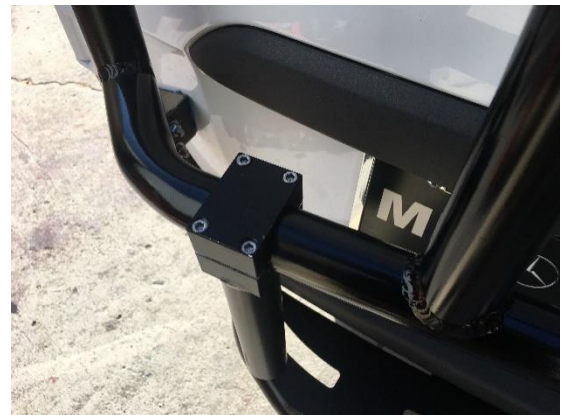
Figure 1: Bolt-On Supports Loosely Bolted to Lower Crossmember
