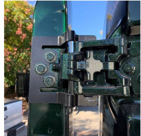
Figure 4: Inside View of Installed Upper Hinge Bracket
