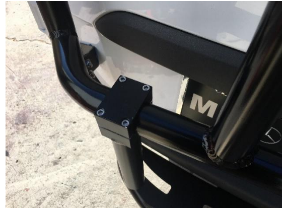
Figure 4: Bolt-On Supports Loosely Bolted to Lower Crossmember
