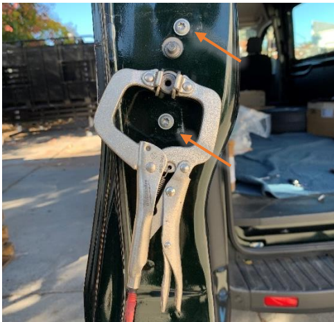
Figure 7: Removing factory torx screws
