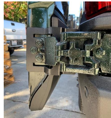
Figure 5: Inside View of Installed Lower Hinge Bracket
