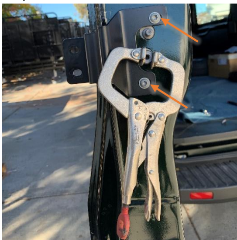
Figure 8: Inner Driver Door Bracket Installed
