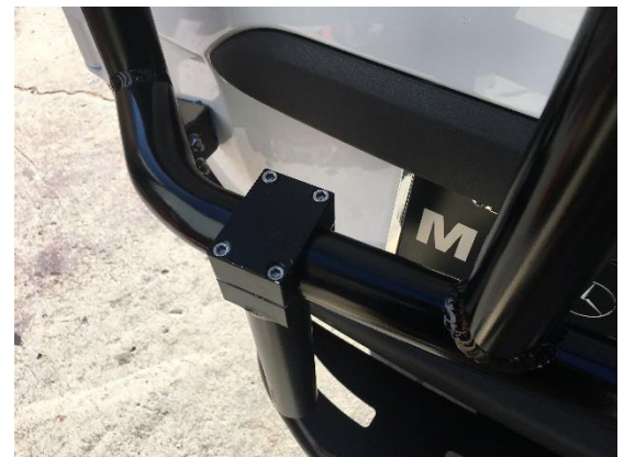
Figure 14: Bolt-On Supports Loosely Bolted to Lower Crossmember
