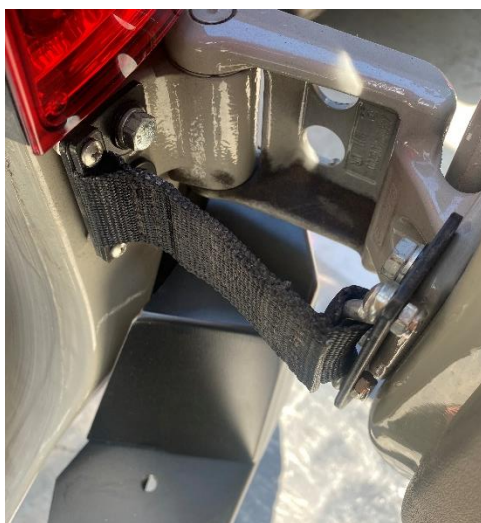
Figure 13: Limiting Strap Installed
