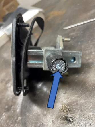
Figure 3: Type 2 Latch Flange Adjustment
