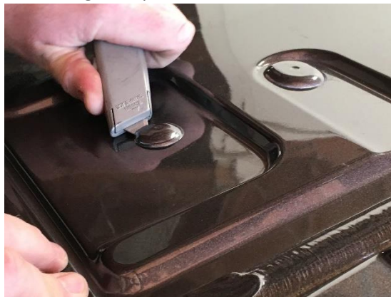
Figure 14: Roof Rack Mounting Point Plug Removal
