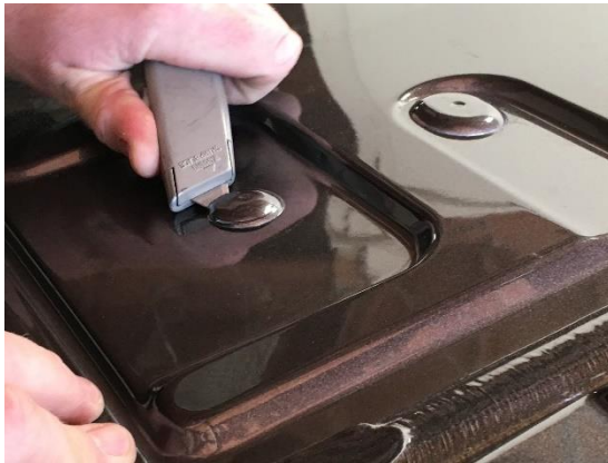
Figure 14: Roof Rack Mounting Point Plug Removal
