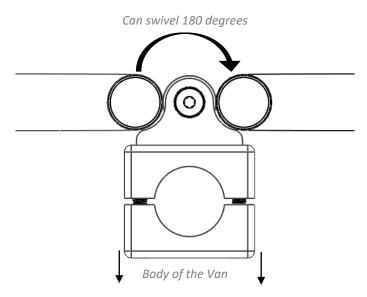
**NOTE:** The tighter the nylock nut is, the stiffer the Surf Hook will be. Adjust the stiffness to your liking, but be sure to not over tighten.
