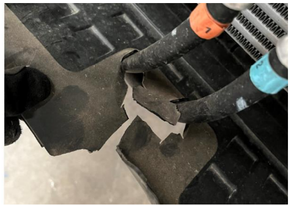
Figure 15: Air Flow Skirt Cut for Removal
