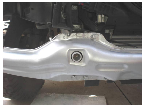
Figure 11: Four (4) Frame Bolts per Side Holding the Stock Steel Bumper to the Vehicle.
