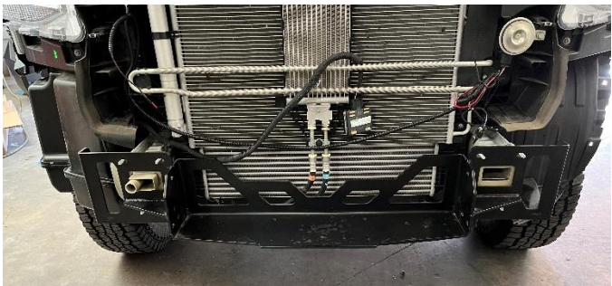
Figure 19: Winch tray Installed
