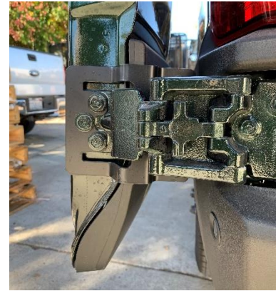
Figure 5: Inside View of Installed Lower Hinge Bracket
