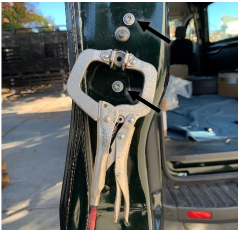
Figure 7: Inner Door Bracket Installed
