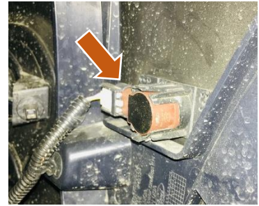
Figure 15: Parking Sensors from Backside of Bumper
