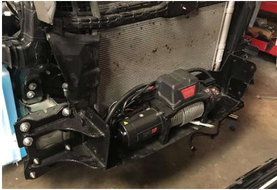
Figure 31: Winch Installed onto Winch Plate
