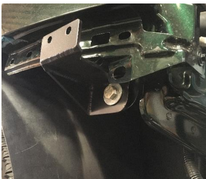
Figure 33: Outer Support Bracket Installed
