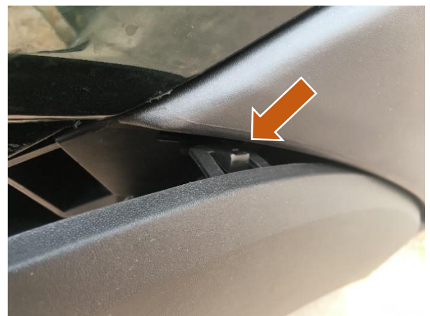
Figure 6: Fender Flare Plastic Clips Catches
