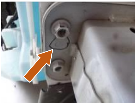
Figure 24: Example of Spot Weld (Shown from the Back)
