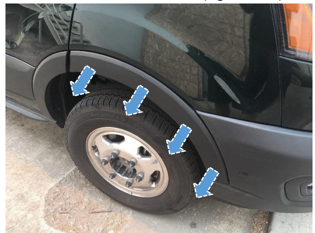
Figure 5: Fender Flare Removal
