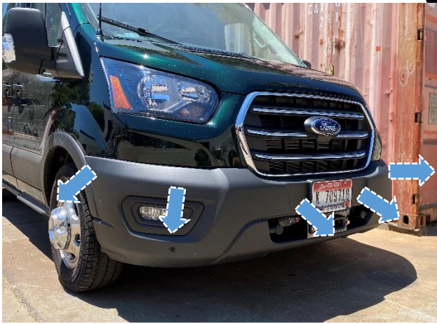
Figure 12: Factory Bumper Removal
