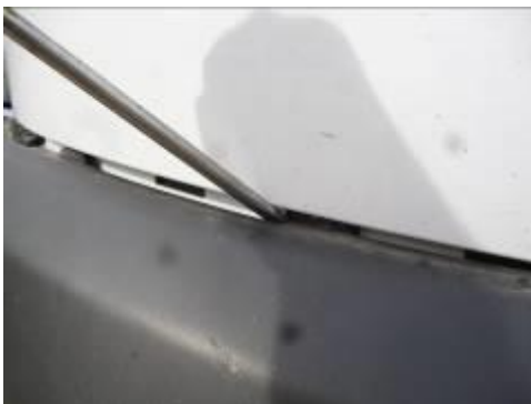
Figure 14: Front Bumper Being Pried from Body
