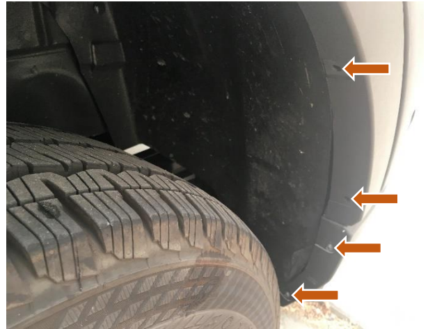
Figure 4: Torx Bolts Along Inner Wheel Well
