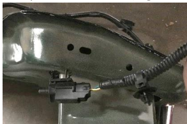
Figure 19: Temperature Sensor Removed
