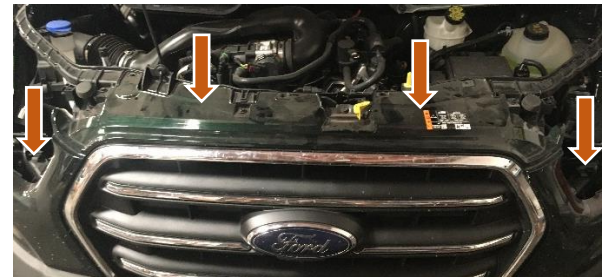
Figure 10: Locations of the Large Plastic Catches
