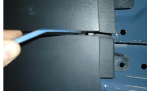
Figure 7: Removing Small Plastic Panel from Rear Bumper
