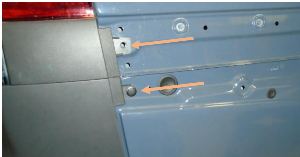
Figure 6: Plastic Rivets Underneath the Side Panel
