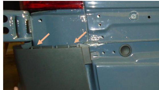
Figure 8: Small Plastic Panel Removed
