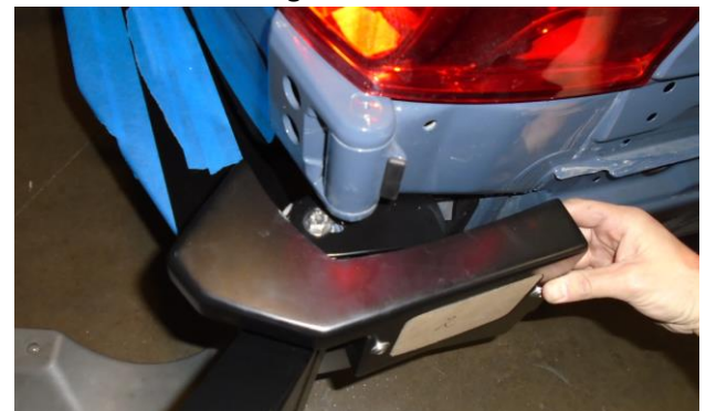
Figure 13: Installation of the Trim Assembly
