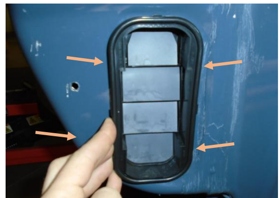
Figure 9: Air Pressure Relief Insert Removal
