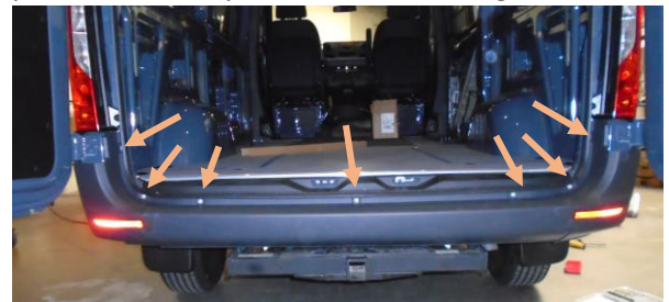
Figure 2: Torx Bolts on the Rear Bumper
