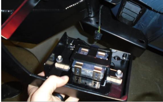
Figure 14: Blind Spot Sensor Installation
