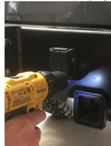
Figure 15: Installation of the trailer plug
