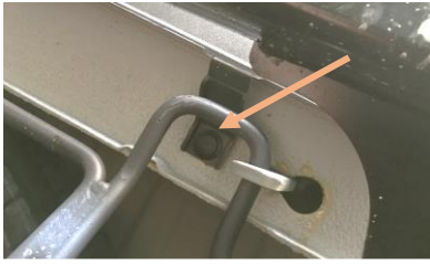
Figure 3: Plastic Rivets Underneath Bumper
