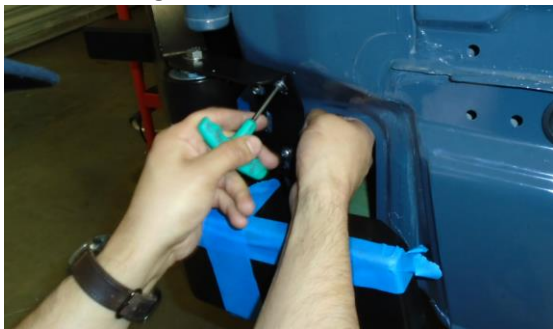
Figure 12: Tightening Hardware Through Insert Opening
