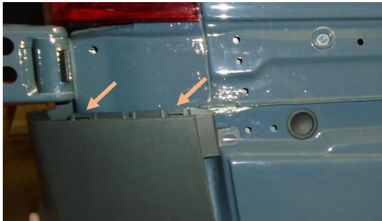
Figure 8: Small Plastic Panel Removed
