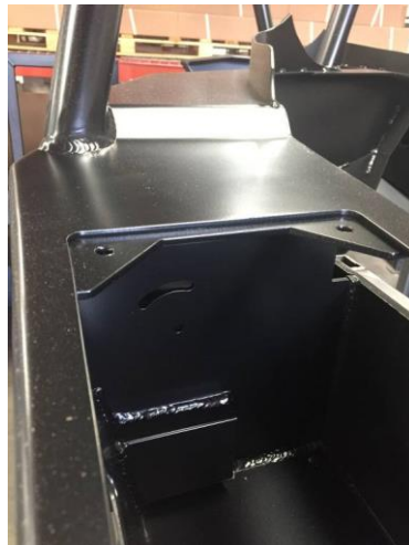
Figure 23. Install the crash sensor bracket in the orientation as shown.
