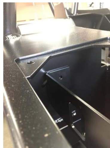
Figure 23. Install the crash sensor bracket in the orientation as shown.
