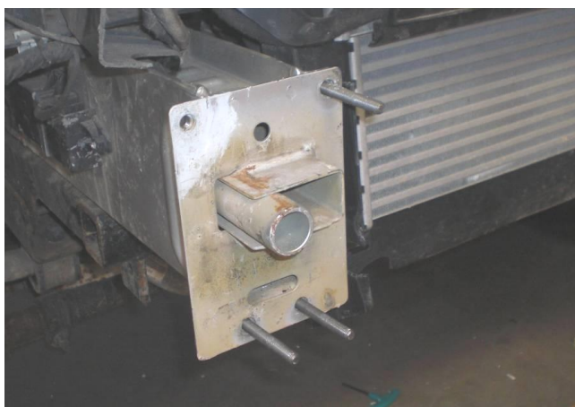
Figure 16: M8 bolts installed on passenger side frame horn
