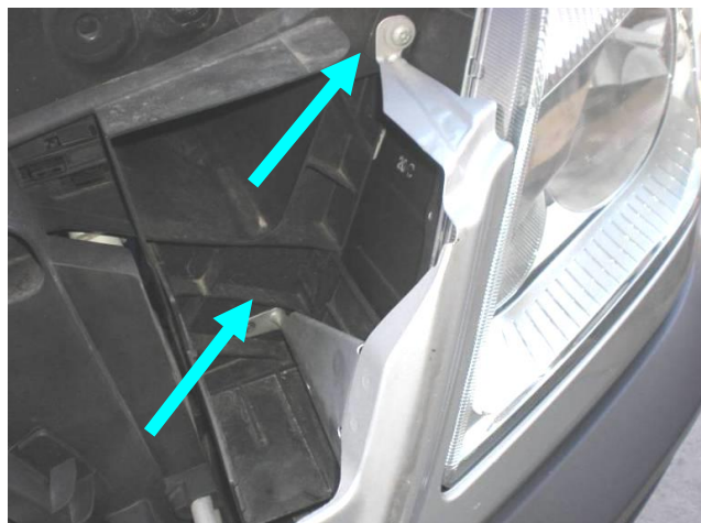
Figure 5: Headlight trim piece torx bolts
