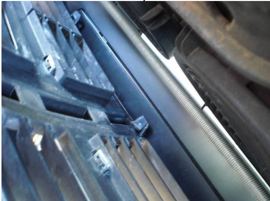
Figure 25: Stock grill installed on Aluminess door tabs
