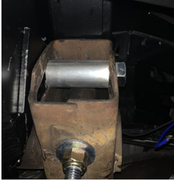
Figure 6: 1/2" hex bolt with crush tube
