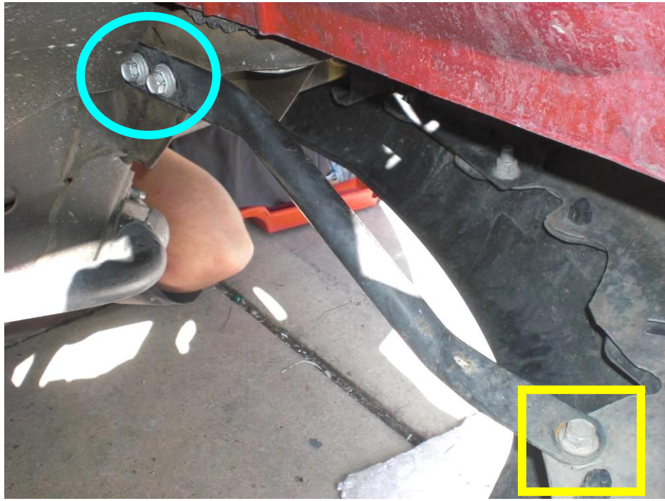
Figure 1: Stock bumper tension rod
