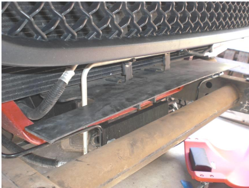
Figure 3: Trimmed plastic shield
